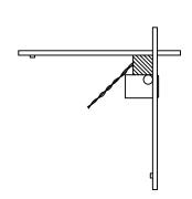
Aerial view of stud and braces. Note that the service lines extend at a 45 degree angle from within the braces
